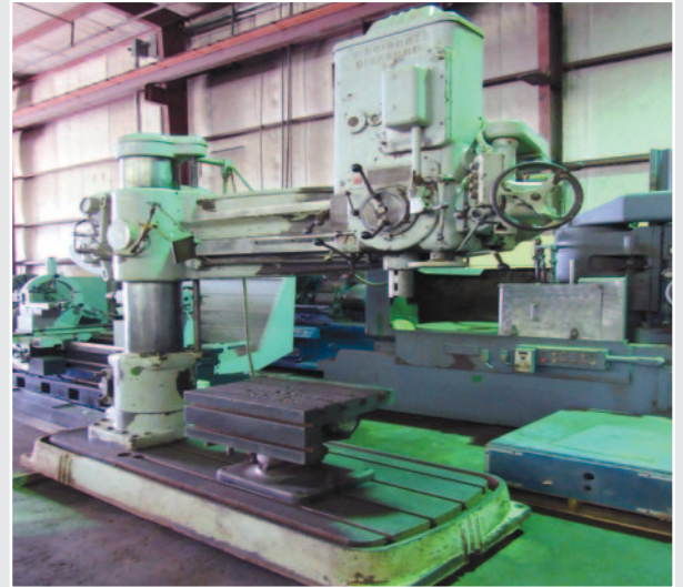
• 4' 13" Cincinnati Bickford Super Service Radial Drill, 48" arm, 13" col., 60" under arm, 21 - 2300 rpm, 10 hp, #5 Morse, 4" spindle dia., 18" spindle travel, tilt box tbl, pwr elev., pwr clamp, rapids, coolant
