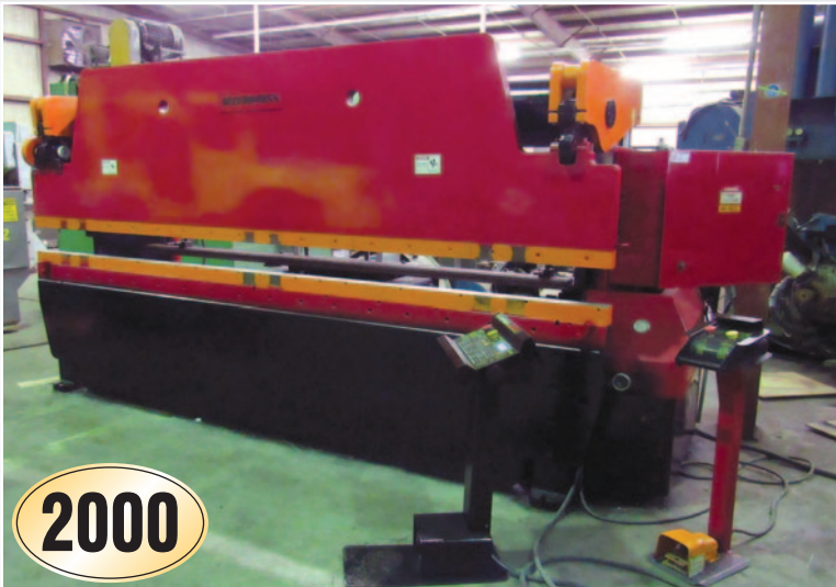
• 100 Ton x 144" Accurpress 710012 Hyd. Press Brake, New 2000, 124" btwn housings, 144" bed length, 8" stroke, 14" open ht., 10" throat, 25 hp, ETS pedestal control, ETS back gauge
