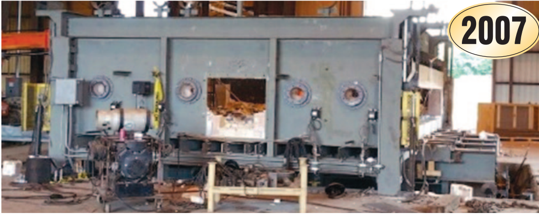
• 2000 Deg. F Plate Furnace w/ Auto Walking Beam Pass Through System , 2007, heat treat plates 48" wide by 20' long and 4-1/2" in thickness
