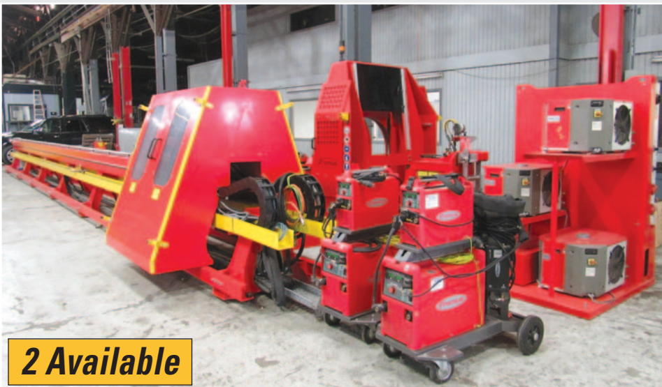
• Fronius I.D. Pipe Cladding Machine, 5' – 42' pipe lengths, 6.6"–36" pipe O.D., 6"–35.4" pipe I.D., HMI-T10 oper. panel, Trans TIG 5000 + Trans TIG 2200 pwr sources, "lights out" operation
