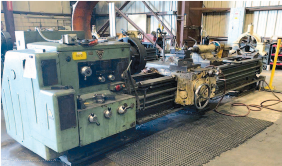
• 26" x 120" Ryazan Engine Lathe, 26" swing, 14" over cross slide, 120" centers, 10 - 1250 rpm, 27hp, 3-3/8" spindle bore, 20" 4-jaw chuck, inch/metric threads, tailstock, taper attach., steady rest, 4-way tool post, chuck guard, coolant
