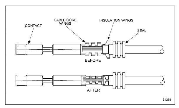
Figure 3-40 Terminal Installation (Shown with a Seal)
