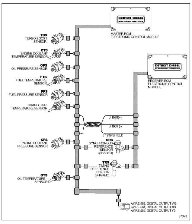
Figure 3-7 A Typical Series 2000 Multi-ECM Engine Sensor Harness
