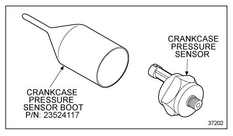
Figure 3-76 Crankcase Pressure Sensor - Series 4000
