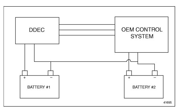
Figure 3-27 Battery System Grounds Connected Using a High Ampacity Cable
