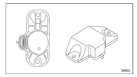
Figure 3-92 The Turbo Boost Sensor - On-highway Applications
