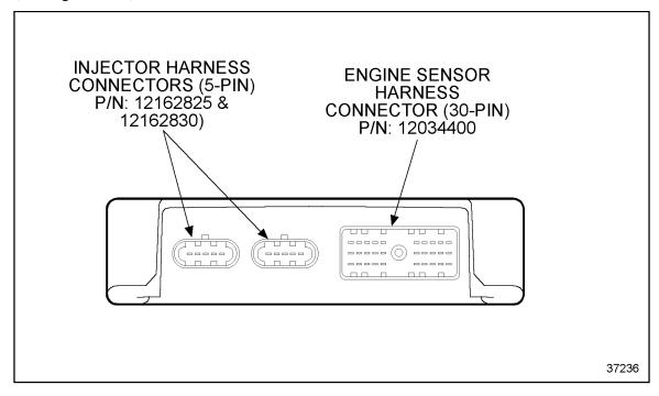
Figure 3-35 ECM Left Side, Engine Harness Connections
