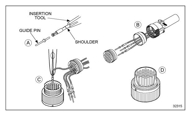
Figure 3-55 Inserting Terminals
