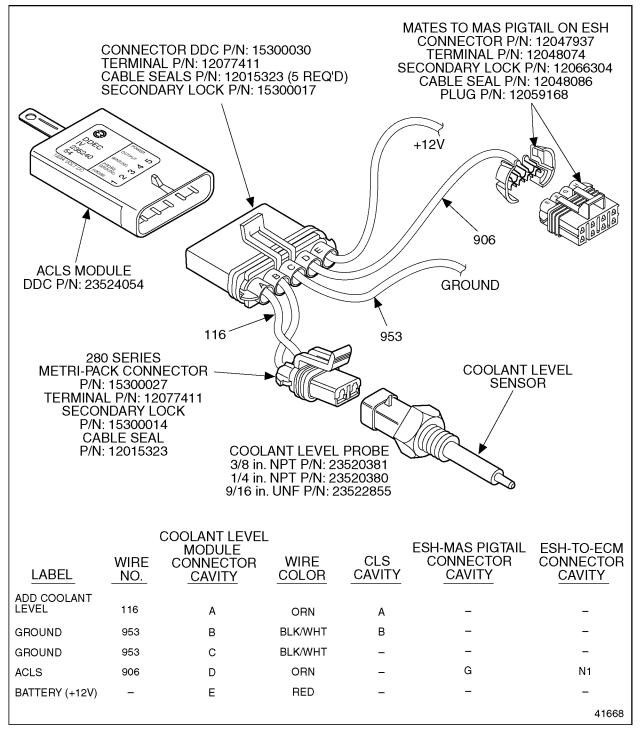
Figure 3-104 Add Coolant Level Sensor Installation
