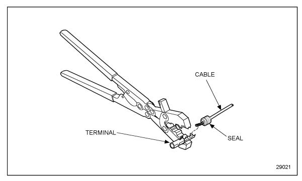
Figure 3-41 Terminal Position (Shown With a Seal)
