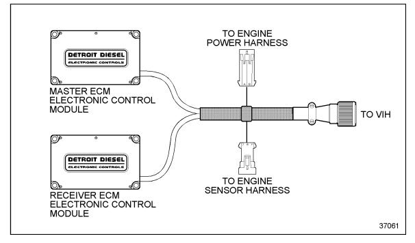
Figure 3-10 A Typical Multi-ECM Engine Interface Harness
