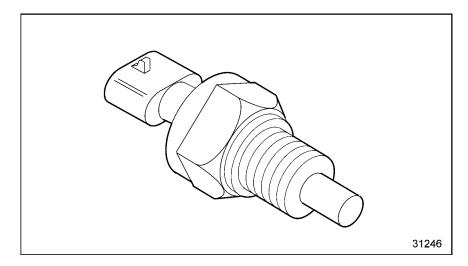
Figure 3-84 Oil Temperature Sensor
