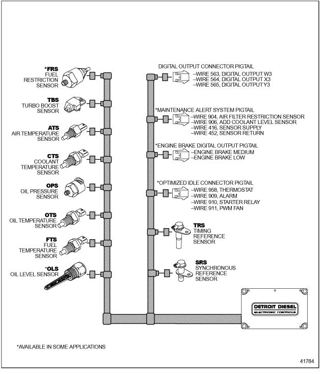
Figure 3-2 A Typical On-highway Engine Sensor Harness
