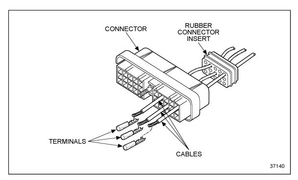
Figure 3-44 Wire Inserted Through the Connector
