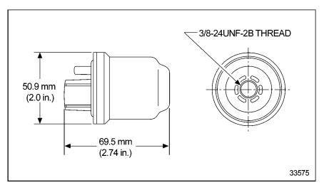
Figure 3-97 Air Filter Restriction Sensor
