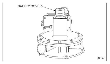
Figure 3-75 Crankcase Pressure Sensor - Series 149
