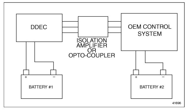
$\Box$  The DDEC circuit must be isolated using an isolation amplifier (see Figure 3-26).
