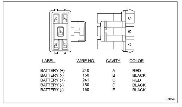
Figure 3-33 Five-Pin Power Harness Connector
