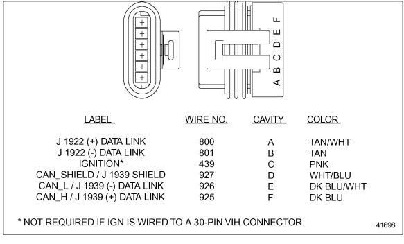
Figure 3-34 Communication Harness Connector
