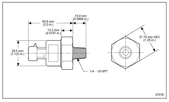
Figure 3-95 Air Compressor Pressure Sensor
