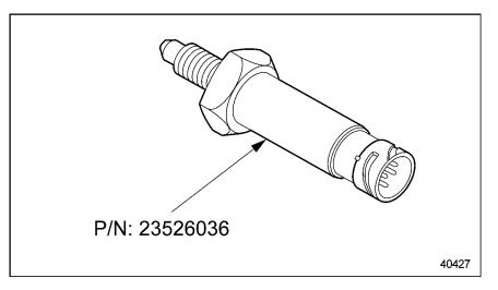
Figure 3-71 Common Rail Fuel Pressure Sensor - Series 4000
