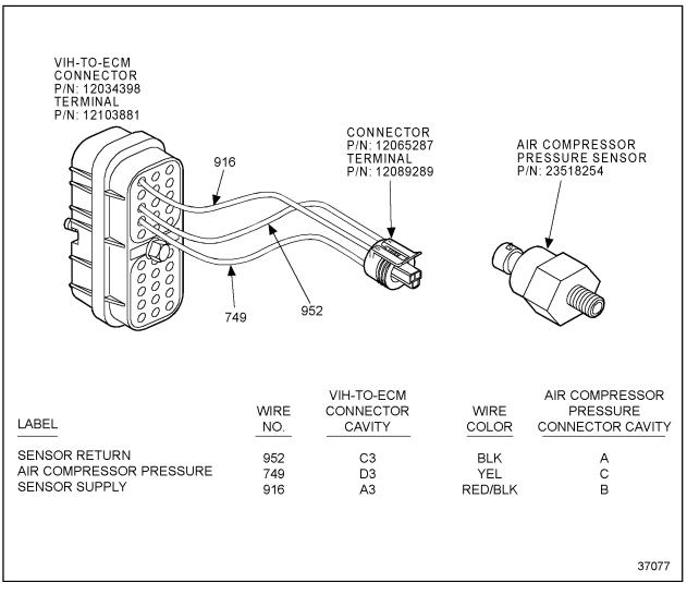
Figure 3-96 Air Compressor Pressure Sensor Installation
