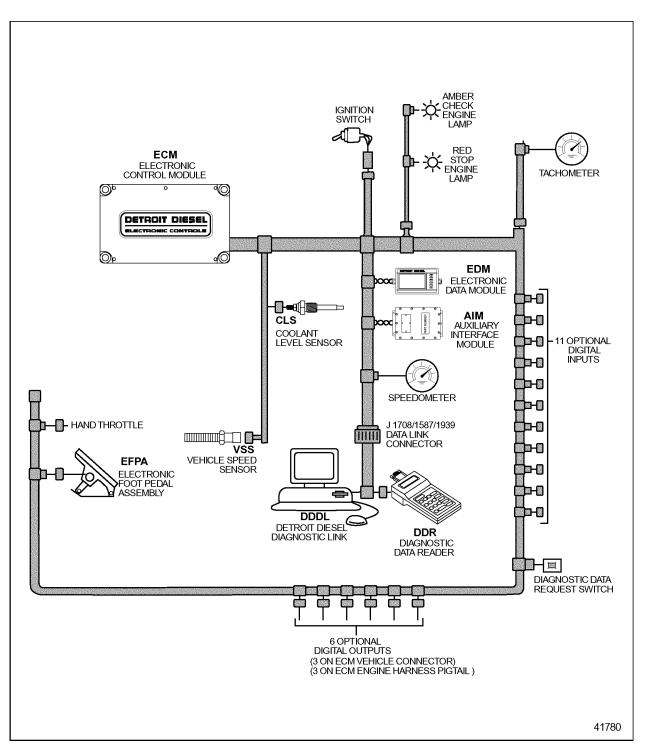
Figure 3-9Typical Construction and Industrial Vehicle Interface Harness
