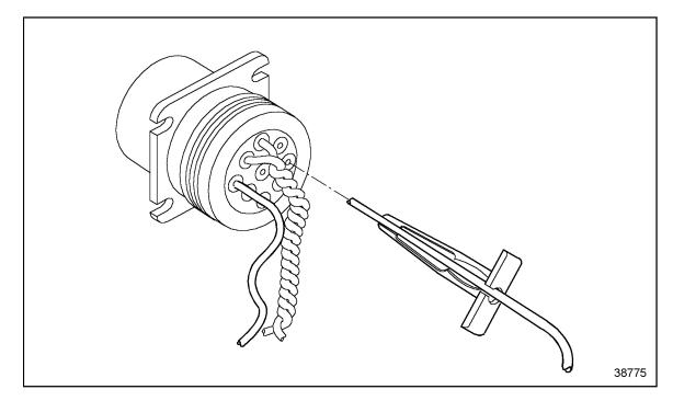
Figure 3-51 Removal Tool Insertion
