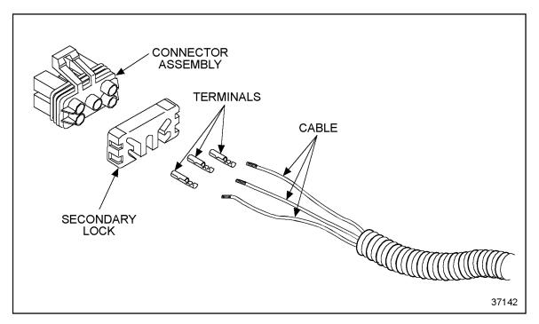
Figure 3-42 Typical Push-to-Seat Terminal Installation
