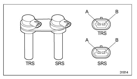
See Figure 3-88 for the Series 92 6/8V, 8V-92, and Series 71 12V engine TRS and SRS.
