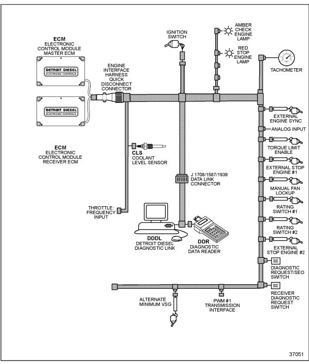
The OEM Vehicle Interface Harness connects to the quick disconnect connector (see Figure 3-11 and Figure 3-12). Refer to Appendix B for a harness schematic.
