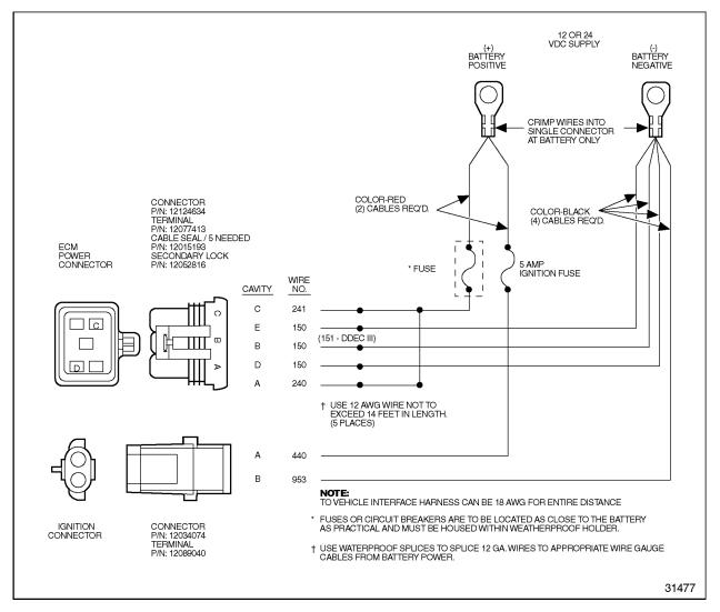
Single fuse installations are simpler and less expensive than two fuse installations. See Figure 3-21.
