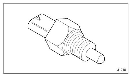
Figure 3-69 Air Temperature Sensor
