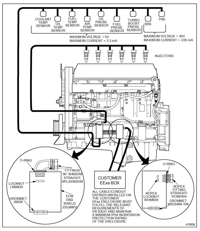
Figure 3-122 Series 50/Series 60 Engine-mounted ECM
