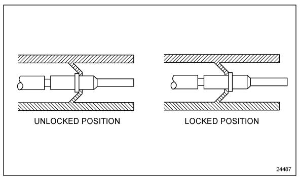
Figure 3-49 Locking Terminal Into Connector
