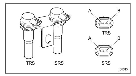
Figure 3-89 The SRS and TRS - Series 71 4/6V Engines
