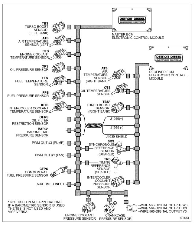
Figure 3-6 A Typical Series 4000 Multi-ECM Engine Sensor Harness
