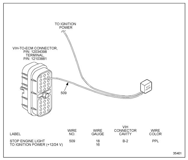
Figure 3-120 Stop Engine Light Wiring
