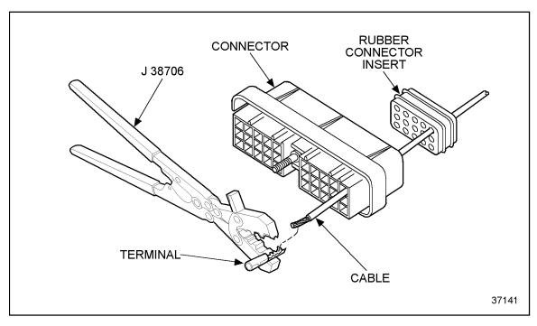
Figure 3-45 Typical Terminal Position
