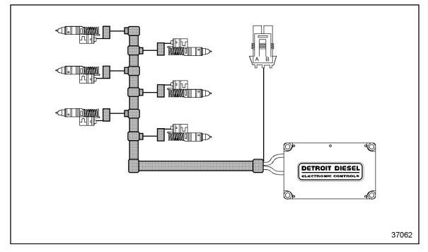
Figure 3-16 Typical On-highway Injector Harness
