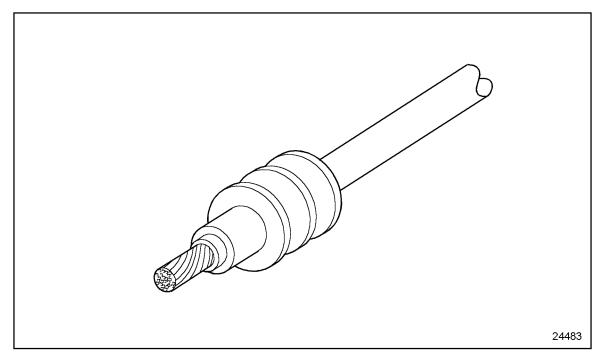
Figure 3-39 Seal Positioning
