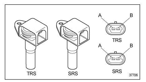
Figure 3-91 The SRS and TRS - Series 53 6V Engine
