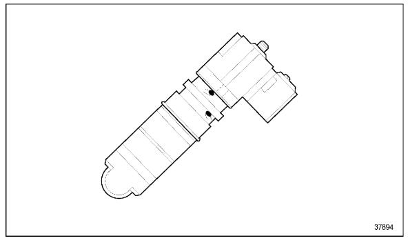
Figure 3-18 Electronic Unit Pump Assembly
