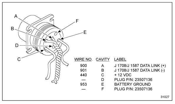
Figure 3-38 Wiring for Six-pin Data Link Connector
