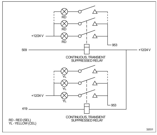
Figure 3-121 Multiple CEL/SEL Configuration - Single ECM Engine
