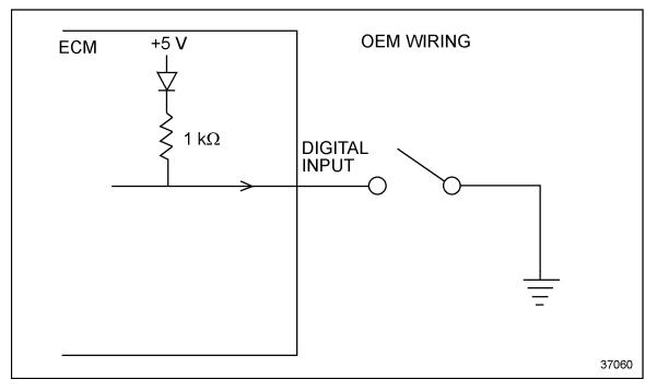
Figure 3-14 DDEC IV Digital Input Circuit
