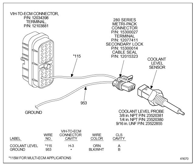
The OEM must connect the CLS probe as shown in the next illustration (see Figure 3-100). Polarity of the ground and signal must be correct for proper operation.
