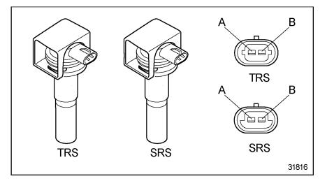
Figure 3-90 The SRS and TRS - Series 149, Series 92 12/16V Engines
