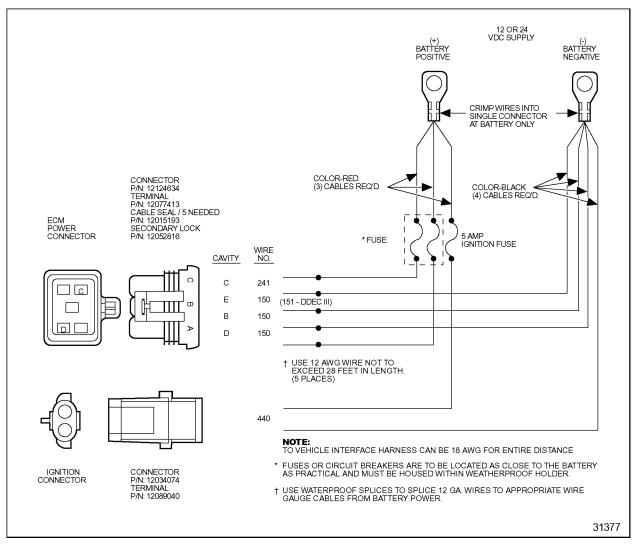
Figure 3-19 Power Harness - Single-ECM, Dual-Fuses
