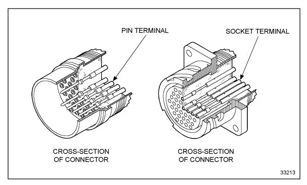
Figure 3-58 Connector Cross-section With Pin and Socket Terminals
