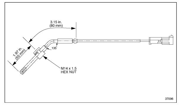
Figure 3-107 Exhaust Temperature Sensor
