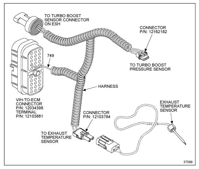
Figure 3-108 Exhaust Temperature Sensor Installation
