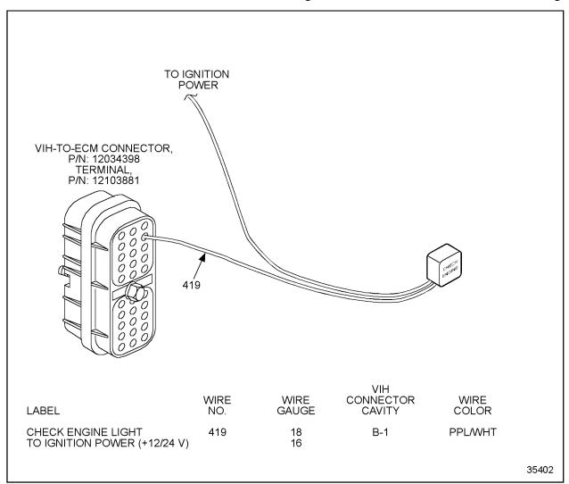
The CEL is connected to wire 419 in the VIH. See Figure 3-119 for the recommended CEL wiring.
