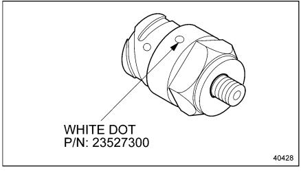
Figure 3-78 Fuel Pressure Sensor - Series 4000
