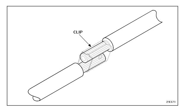
Figure 3-60 Securing the Leads With a Clip
