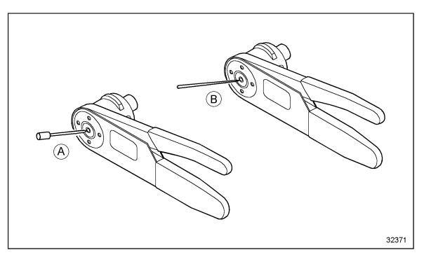
Figure 3-53 Inserting the Terminal and the Stripped Wire.
