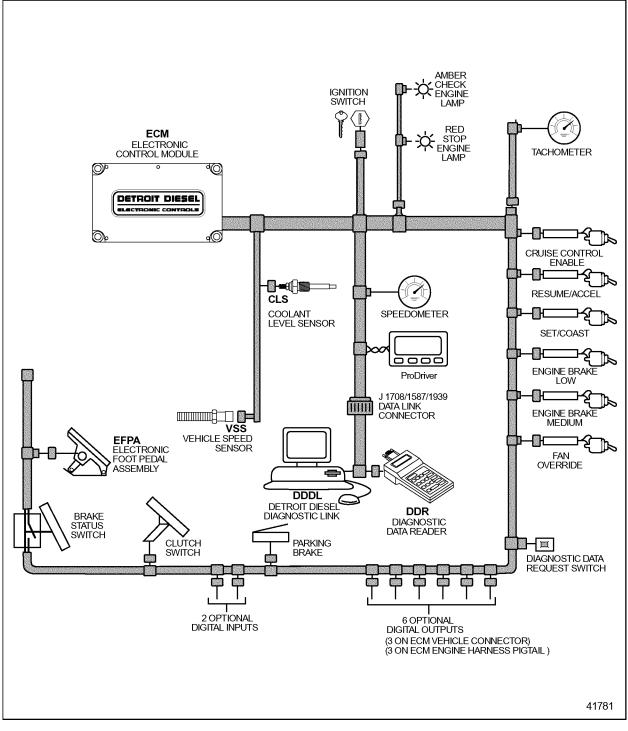
Figure 3-8 Typical On-highway Vehicle Interface Harness
