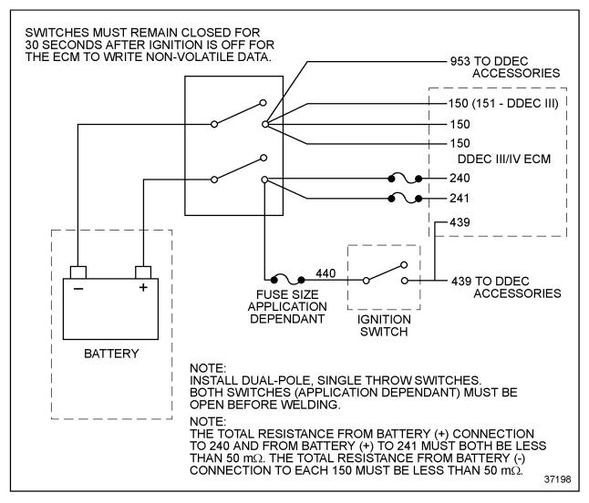
Figure 3-28 Main Power Supply Shutdown 12 or 24 Volt Systems
