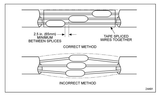
Figure 3-64 The Correct and Incorrect Method of Staggering Multiple Splices
