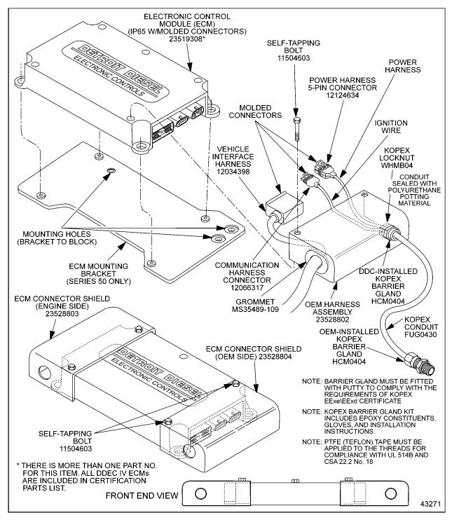
Figures 2:1124 is in Series i50/Series 16000/EM Side OBMnectors, Cables, have shielded to be connected to an EExe junction box.
