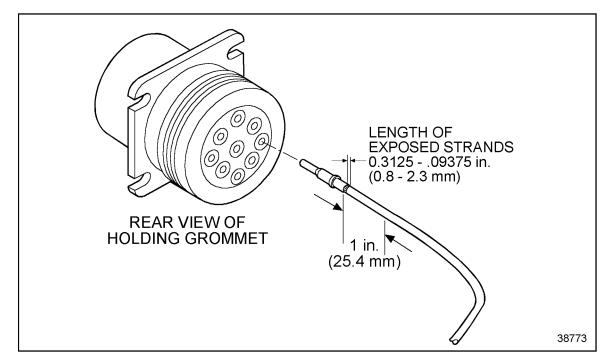
Figure 3-48 Pushing Contact Into Grommet
