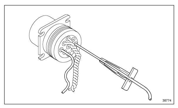
Figure 3-50 Removal Tool Position
