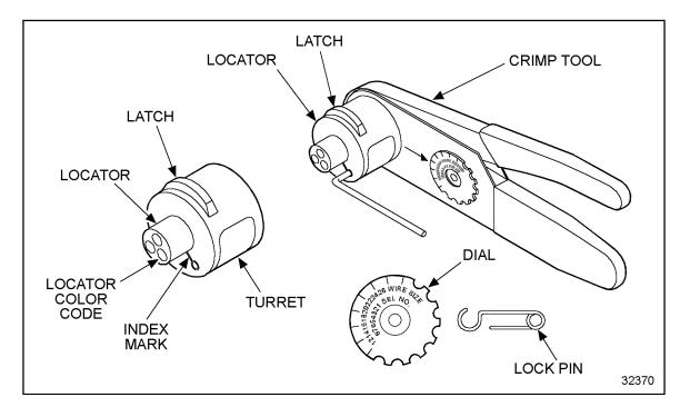
Figure 3-52 Hand Crimp Tool for 37-pin Connector Terminals
