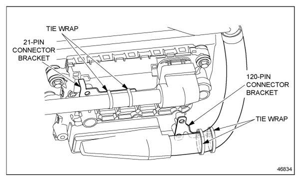
Figure 3-2 Series 60 Engine 120–pin Connector and 21–pin Connector Tie-wrapped to Brackets
