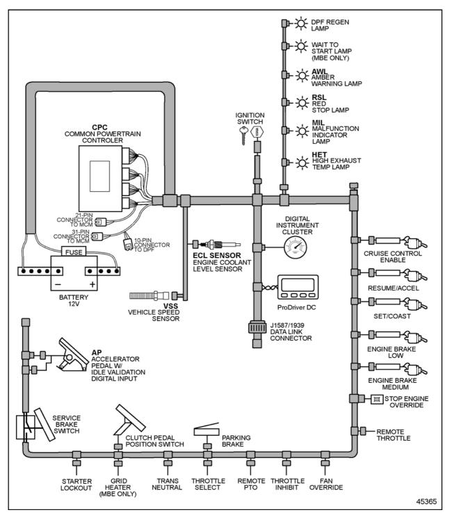
Figure 3-10 Vehicle Interface Harness
