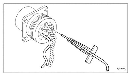
Figure 3-18 Removal Tool Insertion
