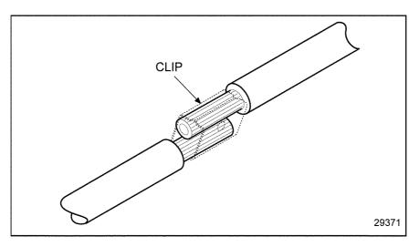
Figure 3-20 Securing the Leads With a Clip
