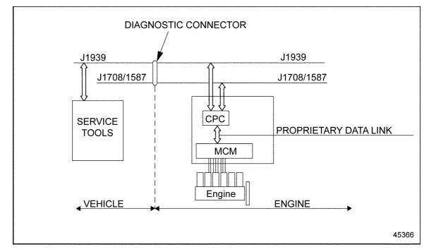
The CPC communicates over the J1587 and J1939 Data Links to the vehicle (see Figure 3-9).
