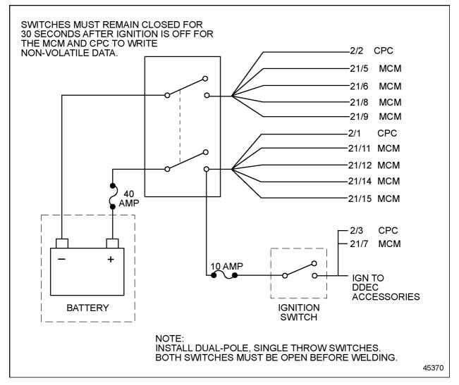
Figure 3-12 Main Power Supply Shutdown
