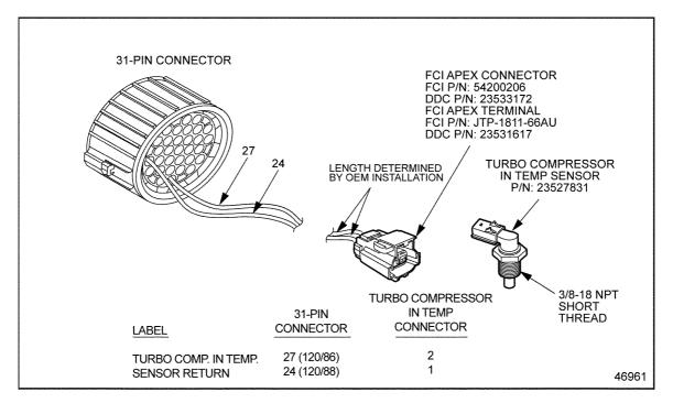
Figure 3-32Turbo Compressor In Temperature Sensor Installation
