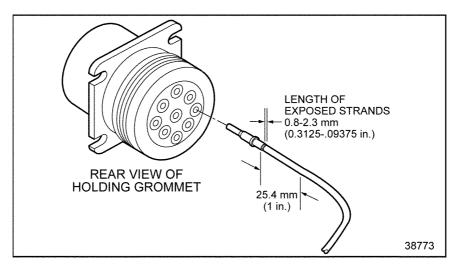
Figure 3-15 Pushing Contact Into Grommet
