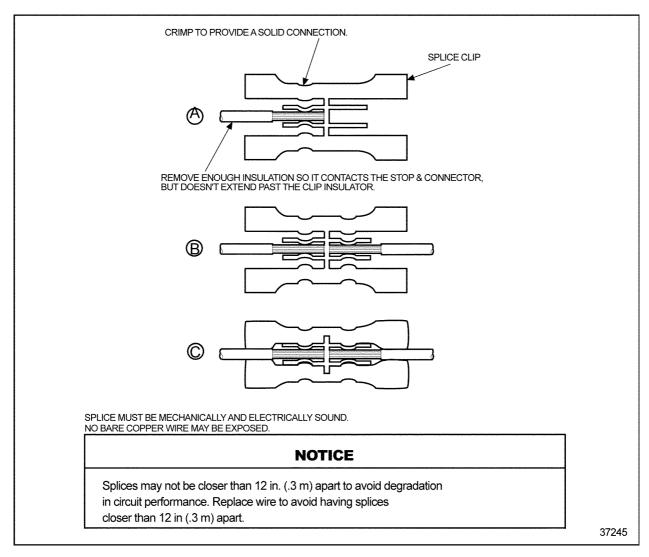
Figure 3-22 Splicing Straight Leads - Alternate Method 1
