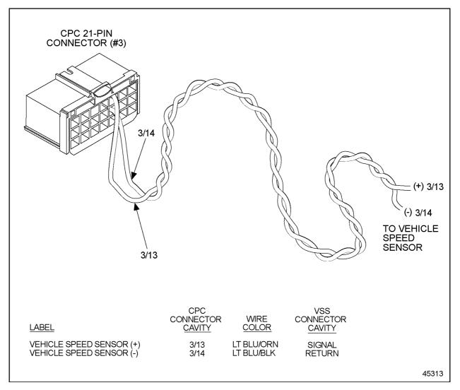
See Figure 3-34 for the installation of the Magnetic VSS.
