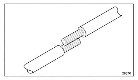
Figure 3-19 Positioning the Leads
