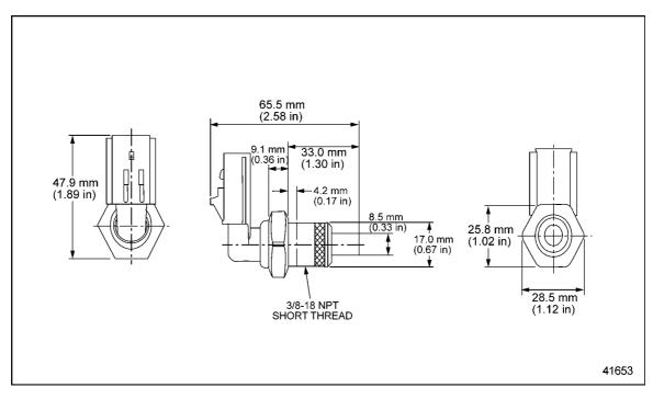
Figure 3-31 Turbo Compressor In Temperature Sensor
