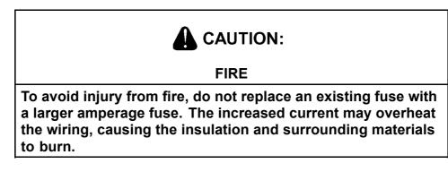
The ignition fuse current rating must be sized for the loads utilized in each application; however, a rating of between 5 and 10 amps is usually sufficient.
