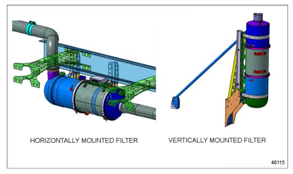
The ATD may be horizontally or vertically mounted depending on the vehicle chassis configuration. See Figure 3-4 for a typical mounting view of the ATD.
