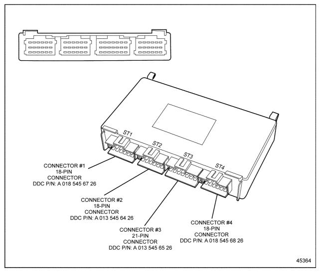
Figure 3-7 The Common Powertrain Controller
