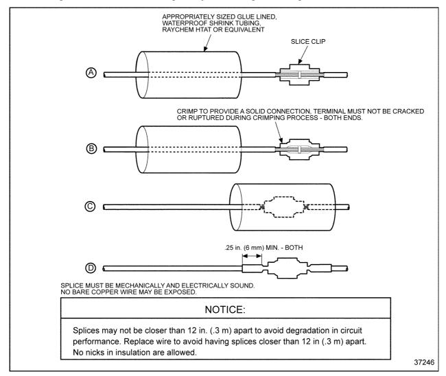
Figure 3-23 Splicing Straight Leads - Alternate Method 2
