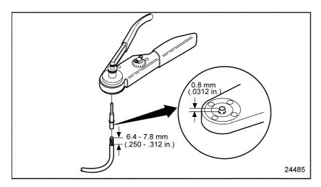
Figure 3-14 Setting Wire Gage Selector and Positioning the Contact
