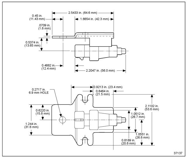
Figure 3-26 Ambient Air Temperatures Sensor Dimensions
