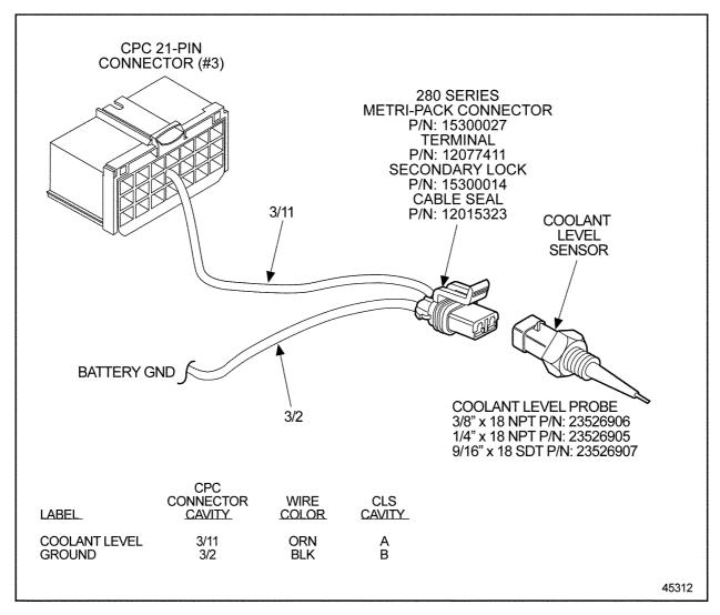
The OEM must connect the ECL Sensor probe as shown in the next illustration (see Figure 3-29). Polarity of the ground and signal must be correct for proper operation.
