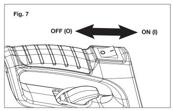
**3.** To stop the unit, press down (O) on the ON/OFF switch, as indicated (Fig. 7).
