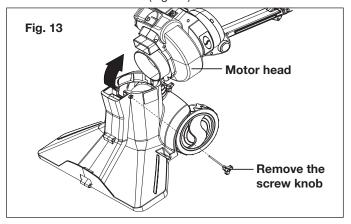
Using protective gloves, carefully remove the material blocking the chute. Inspect to ensure no damage has occurred.
