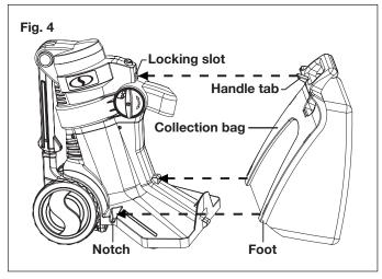
5. Push firmly until the bag clicks into place on the unit body. NOTE: The collection bag must be attached any time the unit is being operated. The unit cannot start if the collection bag is not attached properly.
