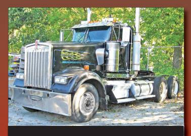
2004 KENWORTH W900 Day Cab Caterpillar C-15/475hp w/engine brake, Eaton Fuller 18 speed transmission, VIT interior, 13,200# front axle, 46,000# rears on air ride suspension, WET KIT, air slide 5th wheel, dual exhaust, 4.11 ratio, 197" w.b.
