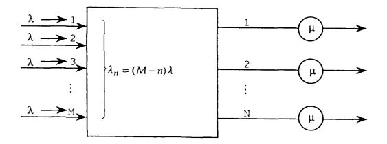
Figure 4. Engset Distribution Model
