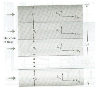
When the flow is parallel to the soil layer, the hydraulic gradient is the same at all points. The flow through the soil mass as a whole is equal to the sum of the flow through each of the
