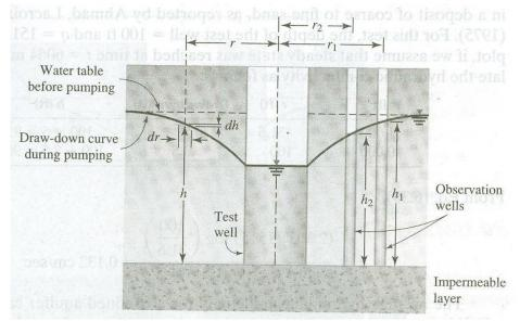
Continuous observations of the water level in the test well and in the observation well are made after the start of pumping, until a steady state is reached. The steady state is established when the water level in the test and observation wells becomes constant.
