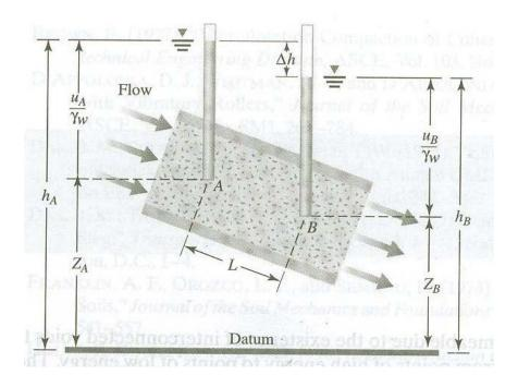
As water flows thorough a soil media as depicted in the figure, there will be a head loss between the two points. This head loss can be given by
