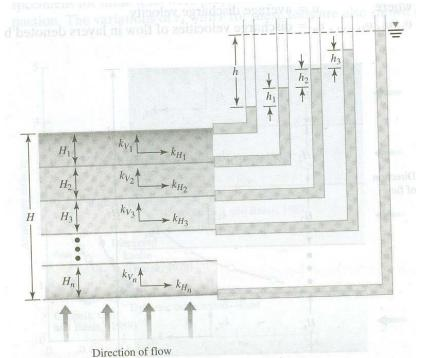
When the flow is perpendicular to stratification, the head loss in the soil mass is the sum of the head losses in each of the layers. The velocity of flow through all the layers is the same. The analogy to electricity is flow of current through resistors in series.
