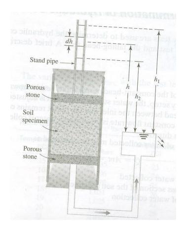
During this test water from the standpipe flows through the soil. The head of water (h) changes with time as flow occurs through the soil. At different times the head of water is recorded. Let dh be the drop in head over a time period dt. The velocity or rate of head loss in the tube is
