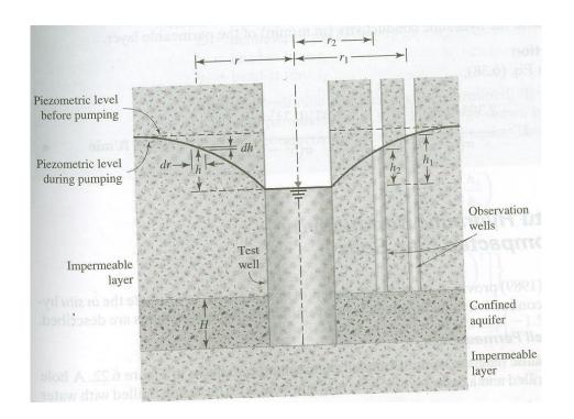
Because water can enter the test well only from the aquifer of thickness H, the steady state of discharge is
