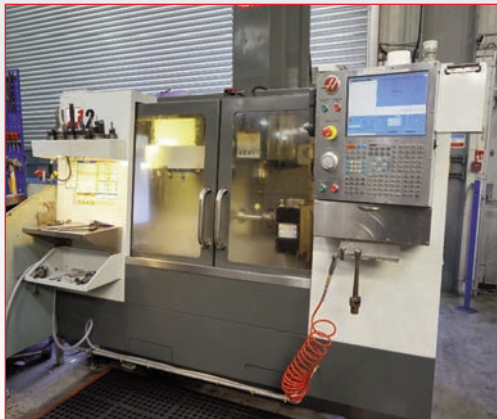
• HAAS VF2 4-Axis Vertical Machining Centre with HAAS CNC Control (2010)
