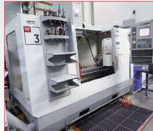
• HAAS VF3 4-Axis Vertical Machining Centre with HAAS CNC Control (2007)
