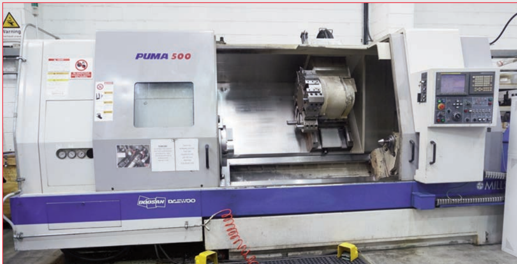
• Doosan Puma 500 Turning Centre with Fanuc 21i TB Control System (2006)
