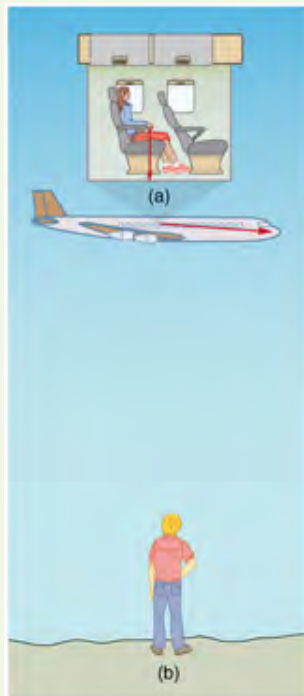
Figure 3.50 The motion of a coin dropped inside an airplane as viewed by two different observers. (a) An observer in the plane sees the coin fall straight down. (b) An observer on the ground sees the coin move almost horizontally.
