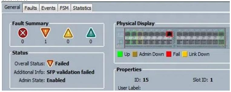
Refer to the exhibit. When an engineer inserts 8-Gb FC SFP port 15 on a Cisco UCS Fabric Interconnect, the port fails. What is a possible cause of the issue?
