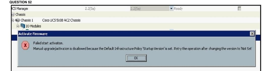
Refer to the exhibit. Cisco UCS Manager is being upgraded using the Auto Install feature, but the FSM fails. Which action resolves the issue?
