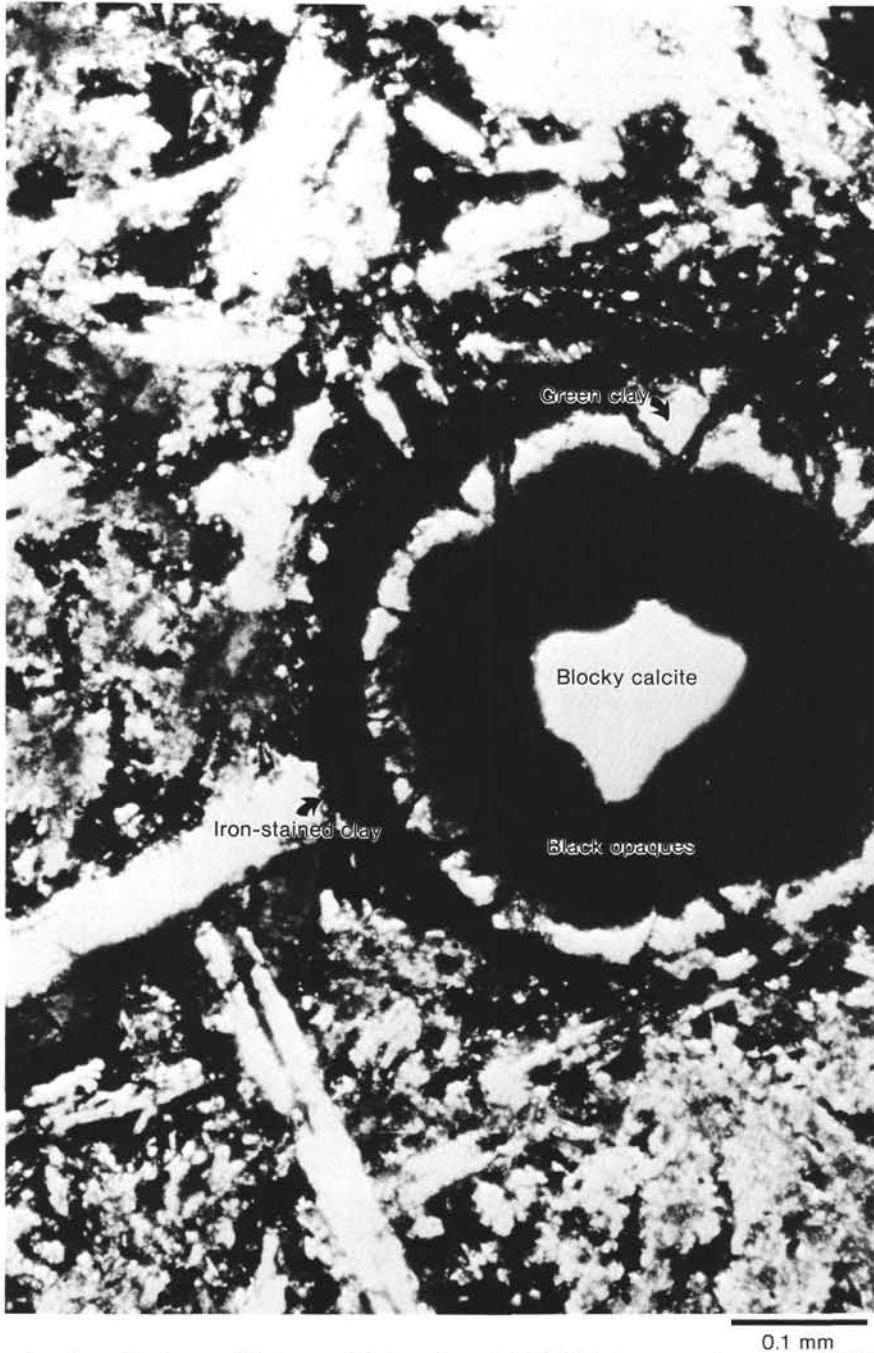
Plate 2. A clay-, opaque mineral-, and carbonate-filled amygdale from Sample 597C-3-1b demonstrating sequential infilling by (1) light green, birefringent clay, (2) black opaque minerals, and (3) blocky calcite. Late-stage iron staining of the amygdale rim blends into groundmass that is pervasively altered and replaced by carbonate and minor zeolite.
