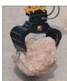
**Multi-Processors.** Thanks to its single basic housing design, the multi-processor series of hydraulic demolition equipment makes it possible to use a range of jaw sets that can handle any demolition job. The multi-processor is the most versatile demolition tool on the market.
