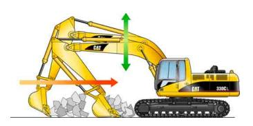
**Rock Scraping.** Scraping rock and finishing work is easy and fast. SmartBoom<sup>™</sup> simplifies the task and allows the operator to fully concentrate on stick and bucket, while boom freely goes up and down without using pump flow.
