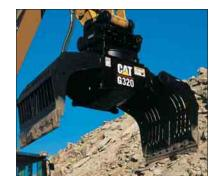
**Multi-Processor.** The Caterpillar Multi-Processors can be equipped with different jaw types depending on your need.
