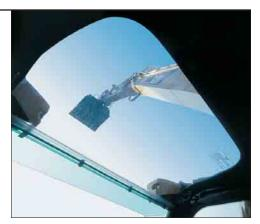
**Skylight.** A unique large polycarbonate skylight provides very good upward visibility, especially usefull in above ground applications.
