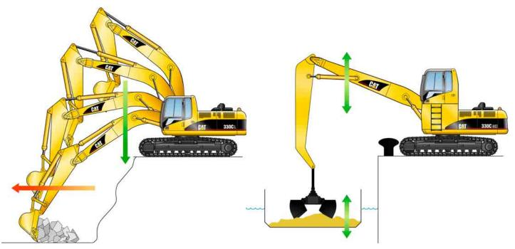
**Truck Loading**. Loading trucks from a bench is more productive and more fuel efficient as the return cycle is reduced while the boom down function does not require pump flow.
