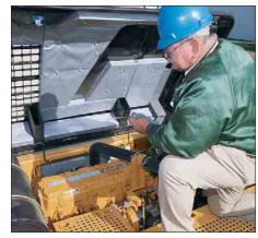
**Engine Inspection.** Engine can be accessed from the upper structure or from under the machine. The engine and pump compartment are separated by a steel fire wall.
