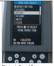
**Electronic Control System.** Ten hydraulic pump flow and pressure settings can be preset, eliminating the need to adjust the hydraulics each
