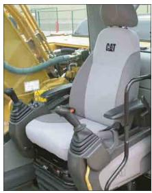
**Consoles.** Redesigned consoles feature a simple, functional design to reduce operator fatigue, ease of switch operation and excellent visibility. Both consoles have attached armrests with height adjustments.
