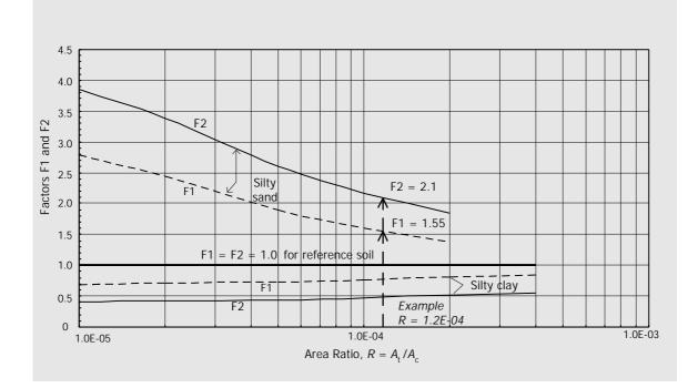
Design Chart 34.A2 Soil Type Adjustment Factors for Trap Area and Sediment Volume
