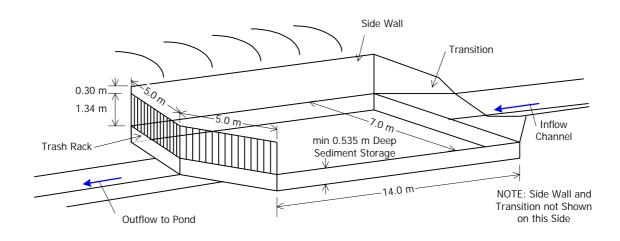
Figure 34.D1 Diagrammatic Layout of Proposed Type 1 SBTR Trap for Sg. Rokam example
