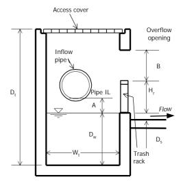
Figure 34.7 GPT Type 2 Trap Dimensions
