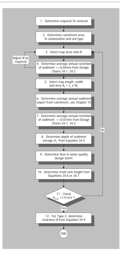
Figure 34.6 Flowchart for SBTR Trap Size Calculation
