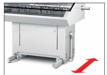
Sliding device for changing the spindle filler tubes on the lathe
