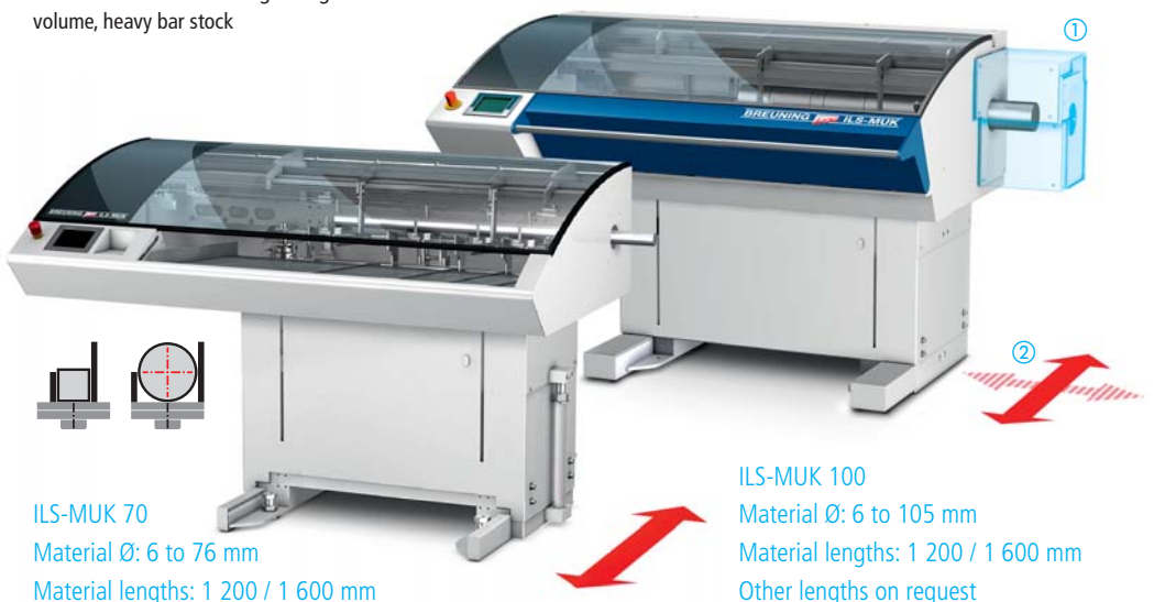
ILS-MUK 100 for the feeding of large-volume, heavy bar stock
