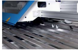
Indexed conveyor for magazing the material bar profiles in a defined position
