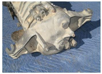
The fourth version of the 901 is commonly known as the "914 Sideshift" transmission, also cast in magnesium and was used from 1973 to the end of 914 deliveries in 1976. The 914 Sideshift transmission was only available in a 5-speed version.
