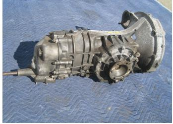
The second version of 901, commonly known as the "911 transmission", is an all-magnesium casting that was used in the rear engine cars (911 & 912) from late in 1968 through the end of 1971. The 911 transmission was available in 4- or 5-speed versions. You will require a 5-speed version to have all the parts needed
