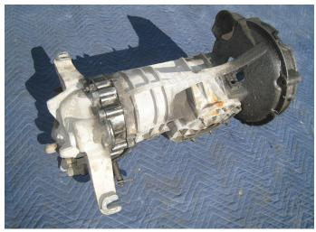
The third version of 901 is commonly known as the "914 Tailshift" transmission that was cast in magnesium and used in the first editions of 914-4 and 914-6 cars during 1970 thru 1972. The 914 Tailshift transmission was only available in a 5-speed version.
