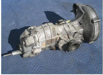
The first version of 901, commonly known as the "Chilled Cast" version, is an all-aluminum casting used in the rear engine cars (911 & 912) from 1965 to 1968. It was available in both 4- and 5-speed versions. You will require a 5-speed version to have all the parts needed.
