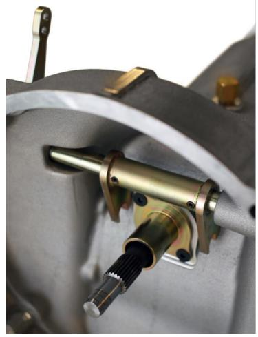
• The release fork is asymmetric, in the area where the bearing is fitted, the thicker finger on the fork should be arranged closest to the transmission, the thin finger closest to the engine.
