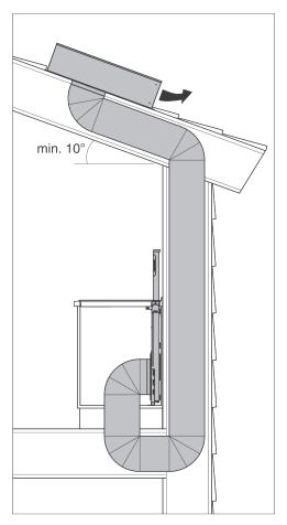
Example: Installation on an external wall Example: Installation on a roof
