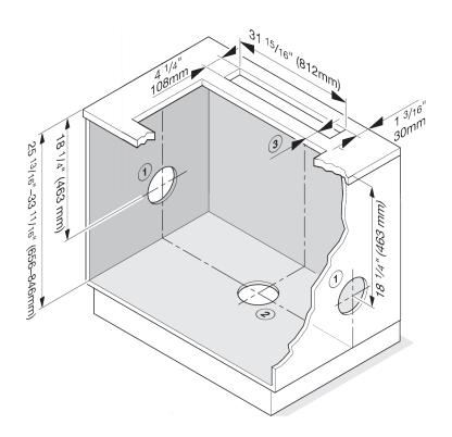
Exhaust or recirculation mode with DAG 600 blower installed at the front of the downdraft. Exhaust ducting ( $\varnothing$  6" (150 mm))
