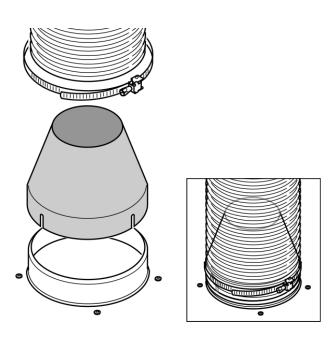
If you would like to reduce the environmental impact of your ventilation system by limiting the CFM output the Reducing Collar can be installed. It reduces the air flow to less than 300 CFM in use with DAG 600. Check local building codes for maximum CFM requirements.
