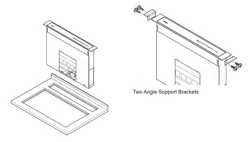
Two small angle brackets are mounted on the downdraft extractor. They serve as a support for the downdraft extractor when the downdraft extractor and cooktop are installed in two separate cutouts.
