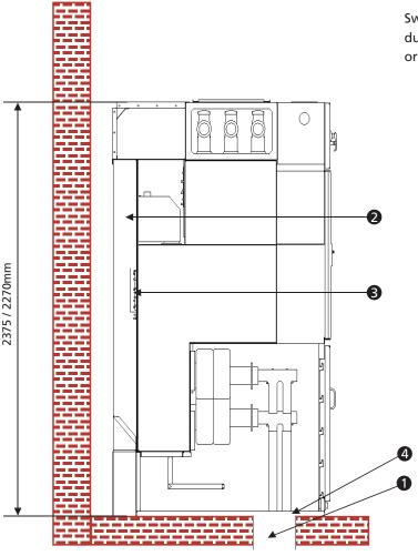
Switchgear installation with rear pressure relief duct (option) for switchgear blocks with IAC A FL or FLR up to 31.5kA/1s
