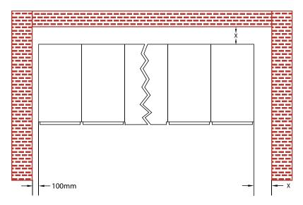
Diagram showing the most compact arrangement of the switchboard line up.
