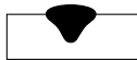
Penetration profile of Argon + Carbon Dioxide shielded GMA weld on Carbon steel
