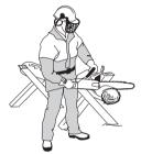
4 Never use the chain saw above shoulder height and avoid cutting with the tip of the bar. Never use the chain saw one-handed!
