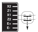
The exciter is switched off by disconnecting the AVR power supply (1 wire on each auxiliary winding) - contact rating 16 A - 250V A.C.
