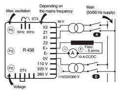
Static adjustment of the current limit, potentiometer P5 (factory setting: 7.5 A, fuse rating: 8 A - 10 seconds).
