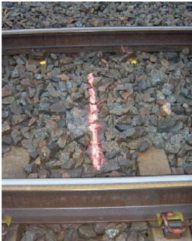
Figure 2.3: Painting line on the ballast during measurements. Any particle displacement has been observed
