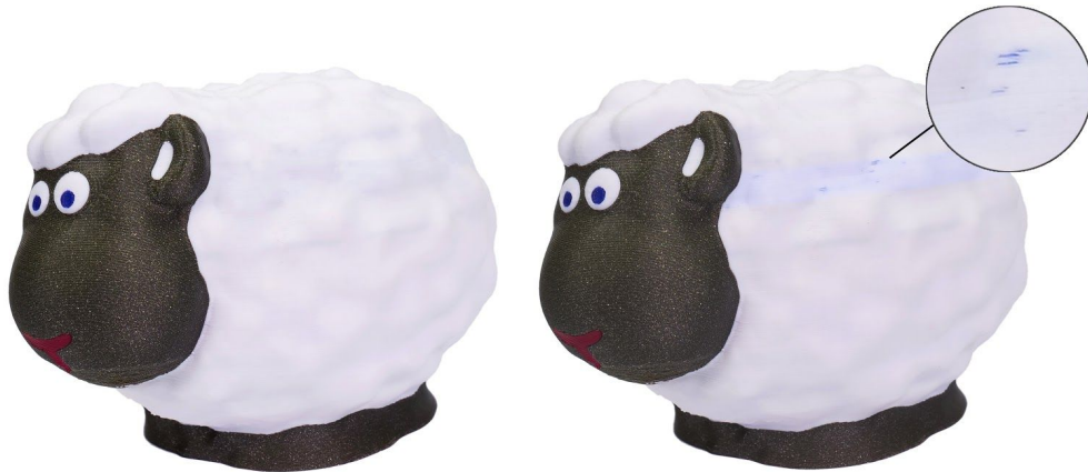
Pict. 21 - Right sheep has contaminated white color due to insufficient purging
