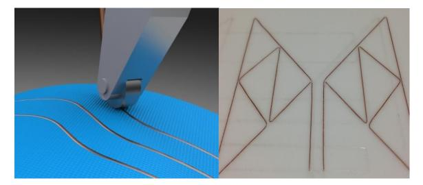
*Figure 2 – Thermally embedded wire (a) conceptual depiction of embedding process and (b) in actual example in a 3D printed substrate (fractal antenna)*
