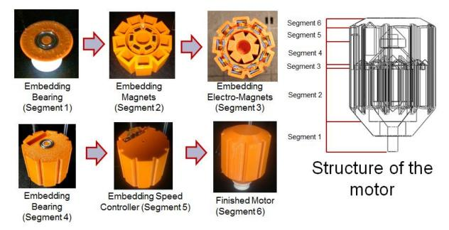
Figure 4 - Pauses in between the build
