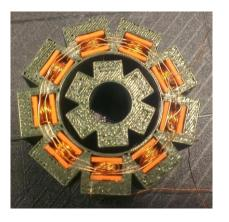
Figure 5 – Electromagnets embedded
