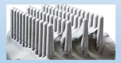
Completed Print with Excess Powder Material attached to Object
