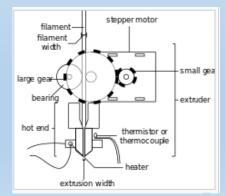
Image 1: Cutaway of extruder and motor
