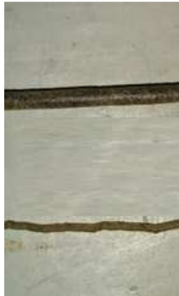
Figure 8. 1.75 mm filament (top) and extruded filament (bottom)
