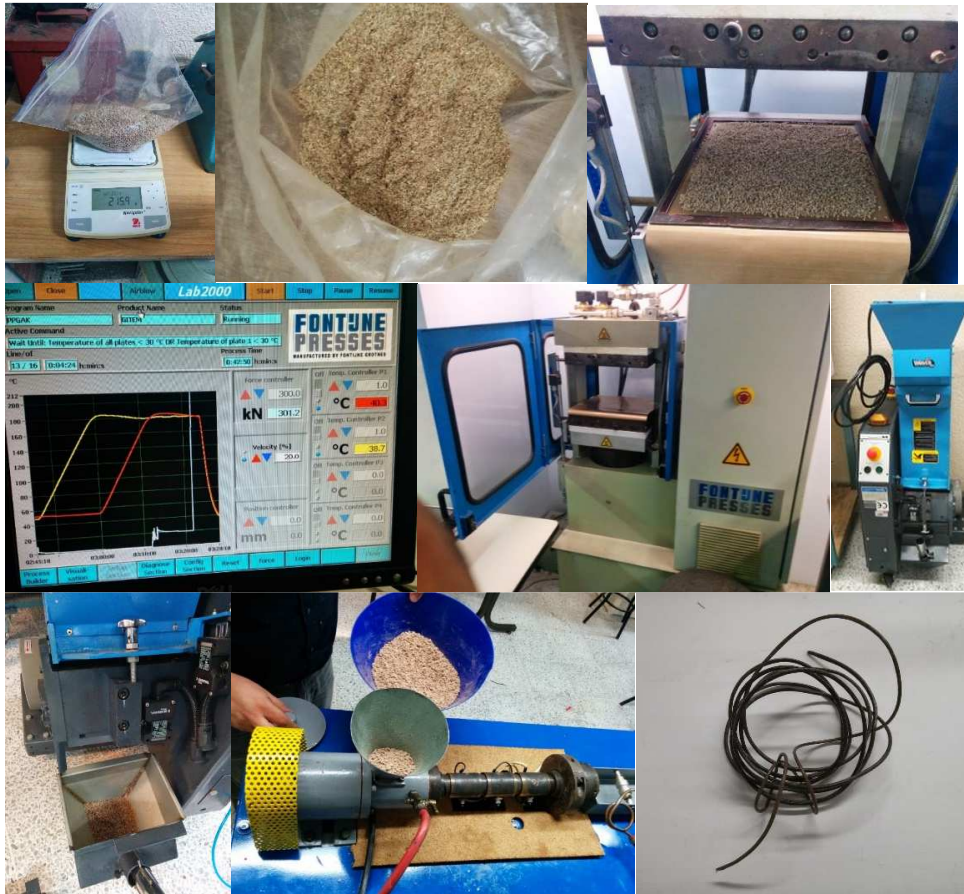
Figure 6. Filament fabrication process.
