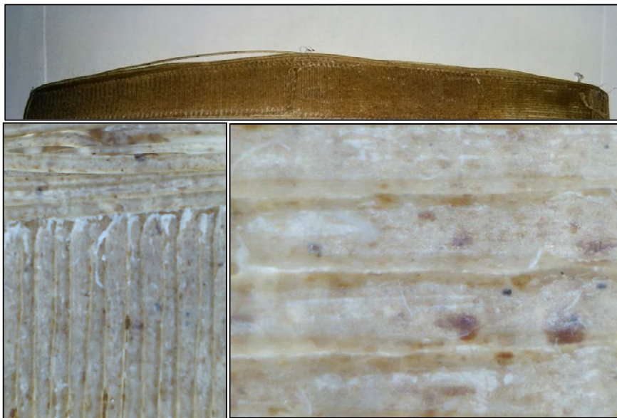
Figure 9. 3d printed sample. (Top). 10x close up (Bottom Left) and 20X (Lower Right)
