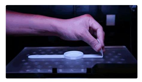
Removal is easy with no spatulas required! Just pull and peel your object right off the build plate!
