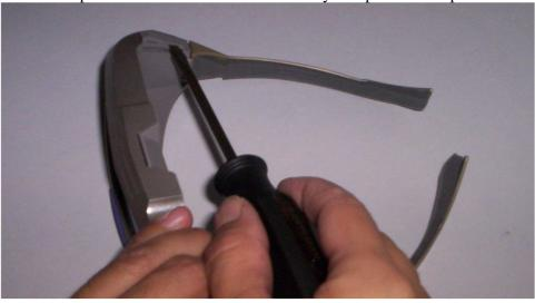
Then move your hand closer to the tip of the screwdriver and pull up changing from the left to right slot. Once the battery compartment is loose then use your hands to remove the battery compartment from the glasses by gently rocking it back and forth.
