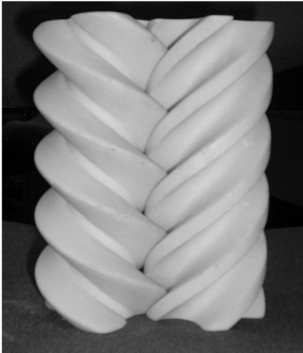
Fig 4.1 Rotors Fabricated by Rapid Prototyping
