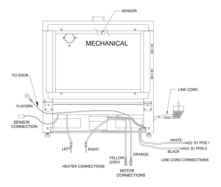
Front View Mechanical Models (Door and Control Panel Removed)
