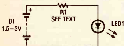
Fig. 2. Here is the simple circuit that comprises the electrical portion of the Electronic Fish Lure. Note: The resistor (R1) may or may not be needed; that will have to be determined by experimentation.
