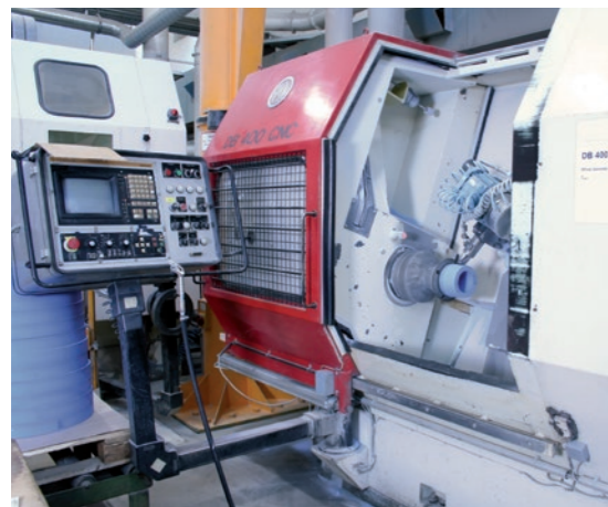
CNC-controlled precision lathes to ensure precise finishing.
