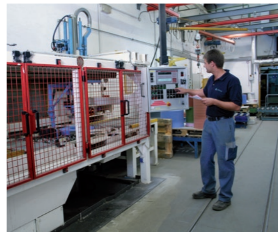
Computer-controlled test machines to test for imbalances and conduct high speed test runs.
