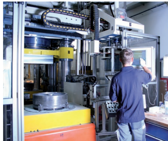
CNC-controlled presses to ensure the homogeneous wheel structure is reproducibly maintained.
