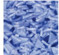
3M Precision-Shaped Grain (Sintered corundum)
