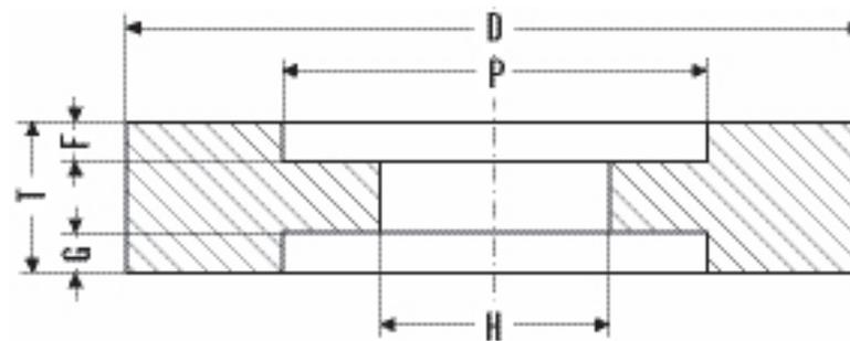
**Caution: The grinding wheel may only be weakened to one half the thickness of the wheel by gouges.**
