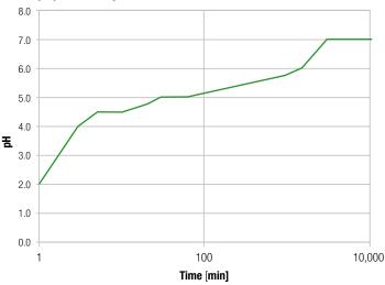
pH profile of RelyX<sup>™</sup> Unicem 2 Automix Self-Adhesive Resin Cement
