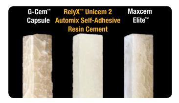
Fig. 18: Results of stress test on self-adhesive resin cements. All samples were self-cured and thermocycled 10,000 times. Source: 3M ESPE internal data
