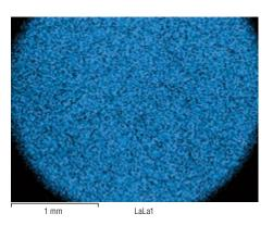
Fig. 16: Element (lanthanum) mapping of a RelyX<sup>™</sup> Unicem 2 sample shows homogeneous distribution over the cement disc surface. Source: 3M ESPE internal data
