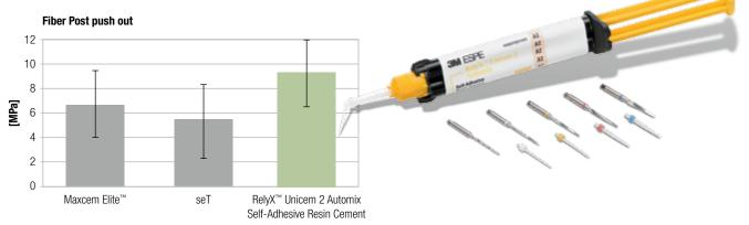
Fig. 11: RelyX<sup>™</sup> Unicem 2 Automix cement exhibited a significantly greater retentive ability and provided a better marginal seal in the root canal than the other self-adhesive resin cements. Source: Interfacial strength and morphology of new self-adhesive resin cements. A. CANTORO, C. GORACCI, A. MAZZONI, L. BRESCHI, and M. FERRARI ; IADR 2010 #621
