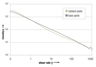
Fig. 15: The catalyst and the base paste show similar behaviour in viscosity when shearing. Source: 3M ESPE internal data
