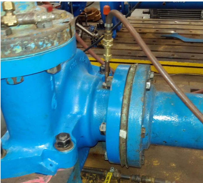
Figure 20: Location of the casing suction tapping.
