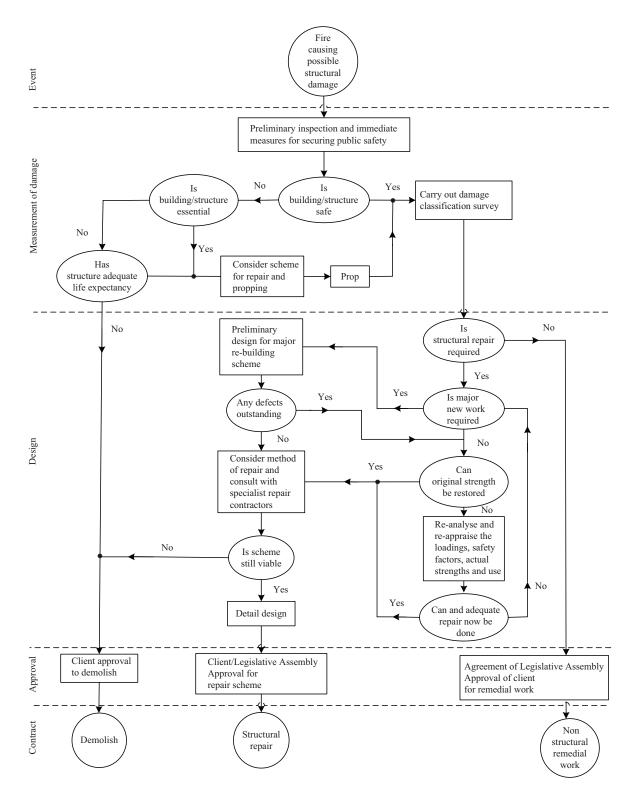
Figure 4.1.2. Appraisal procedure for fire damaged concrete structures, see (Concrete Society 1990).
