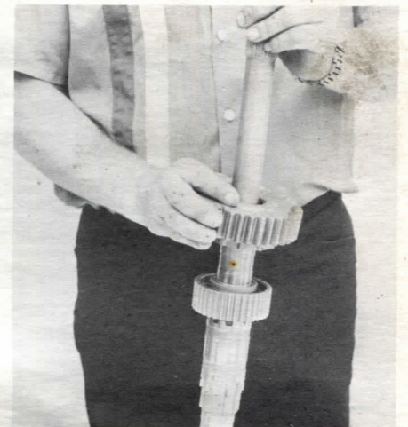
After 1-2 hub is installed, first gear should be placed on mainshaft from rear.
