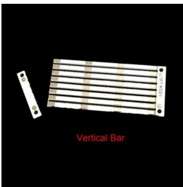
Solder the Vertical PCB to the Horizontal Bar with the LED's soldered on.
