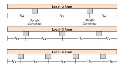
The final item to consider is the width of the product itself. The product should overhang the outside of the arms by some amount. Be careful to not have it overhang too much. We recommend the load should overhang the end arms by one-half the distance from upright centerline to upright centerline. Failure to observe this measure may cause an overload condition on the arms.
