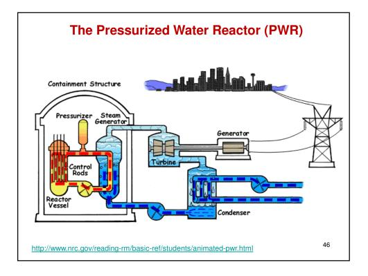
In a **PWR** the primary coolant (water) is pumped under high pressure to the reactor core where it is heated by the energy generated by the fission of atoms. The heated water then flows to a steam generator where it transfers its thermal energy to a secondary system where steam is generated and flows to turbines which, in turn, spins an electric generator. In contrast to a boiling water reactor, pressure in the primary coolant loop prevents the water from boiling within the reactor.
