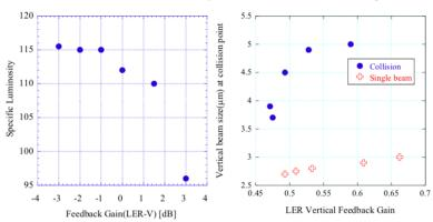
Discovery of luminosity decrease in KEKB collider, function of vertical feedback gain
