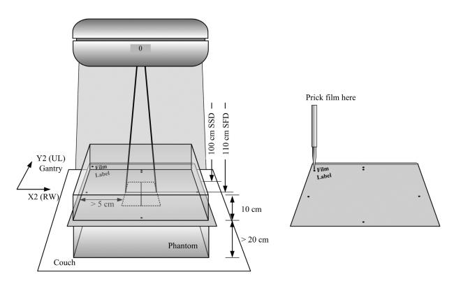
Figure 4.8. Detailed perpendicular phantom setup.
