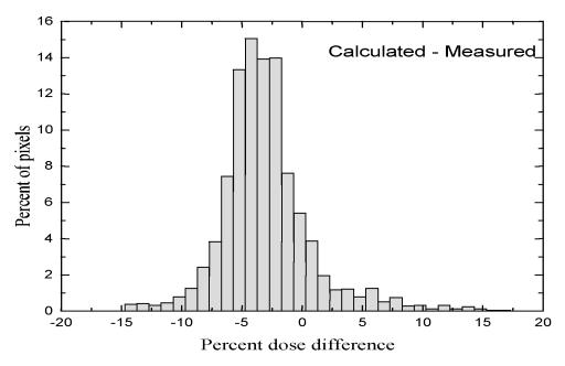
**Figure 4.4.** Dose difference histogram. Assuming the Gaussian distribution, the distribution has a peak at an average value of the distribution. On average, the measured distribution by film overresponds by about 4%, with an uncertainty given by the standard deviation of the distribution (i.e.,  $\sigma = \sqrt{(x_{av})} \cong 2$ , where  $x_{av}$  is the average difference).
