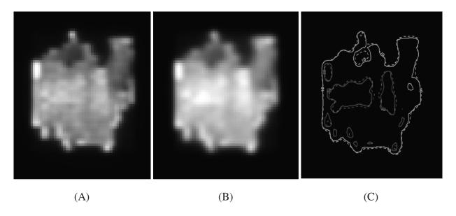
**Figure 4.1.** Comparison of isodose contours (C) from film measurement (A) and RTP calculation (B). A dashed line is for the RTP calculation.
