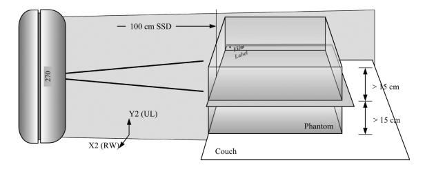
**Figure 4.9.** Detailed parallel phantom setup with gantry and collimator at 270°. Provide additional ±1° to reduce the potential effect of film orientation, if it exists in your setup.
