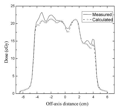
Figure 4.2. Superposition of dose profiles. The film shows overresponse throughout the infield region.
