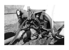
• Prime the pump with water, if needed.
