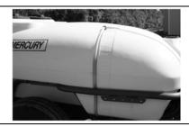
• Fill tank to the correct level and agitate while filling. Continue agitating while driving to the field and whilst spraying unless instructions advise otherwise. If spraying is delayed, agitate thoroughly just before use.
