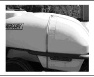
• Fill the tank on level ground per label instructions. If none are given, fill the tank half full with clean water.
