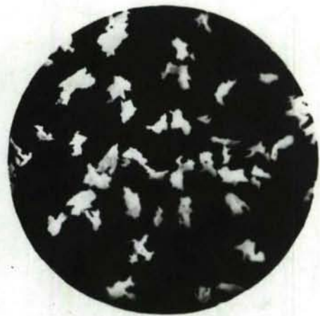
Fig 32 Lead azide co-precipitated with sodium carboxy methyl cellulose (RD1333) X50
