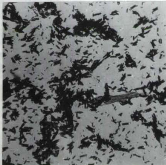
Fig 21 Addition of water dispersed non-ionic surface active agent, 5mins.
