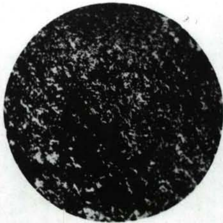
Fig. 25 X50 Lead azide precipitated in the presence of sulphonate type of surface active agent.
