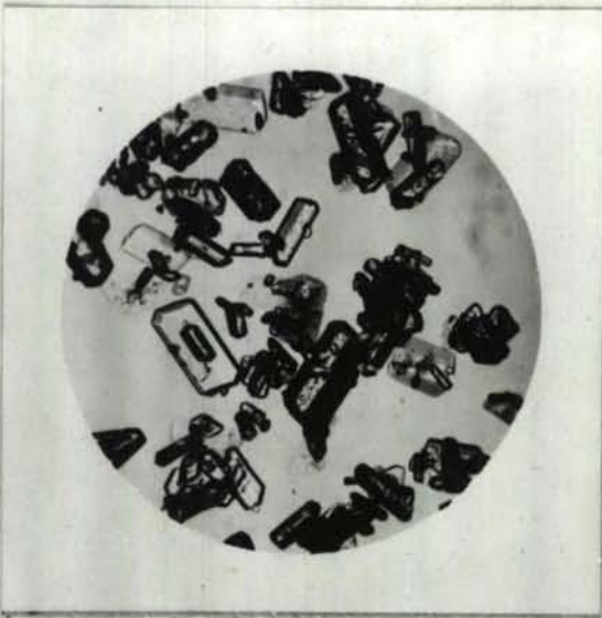
Fig. 1. Barium styphnate from barium acetate and styphnic acid X50
