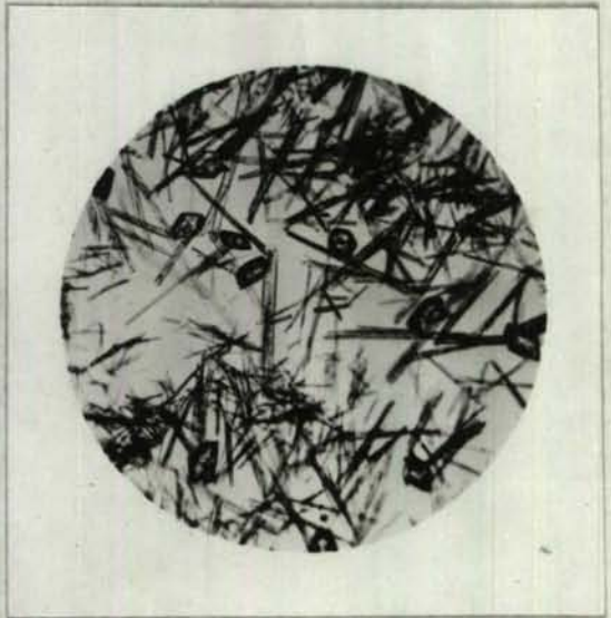
Fig. 6. Barium styphnate trihydrate (accicular) being converted to fig. 5 product (monohydrate). X50
