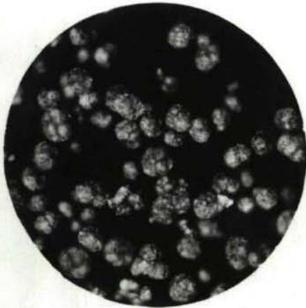
Fig 43. X50 Lead styphnate, granulated, co-precipitated with colloidal graphite
