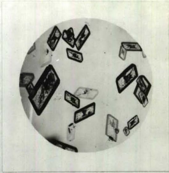
Fig. 2. Barium styphnate from barium chloride added to magnesium styphnate. X50
