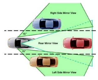
overlap between the inside and sideview mirrors and **allows the driver to monitor the adjacent lane.** Traditional settings overlap with the rearview mirror view and should only be used if the view of the highway from the inside rearview mirror is blocked.
