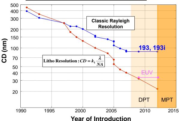
Resolution comes at the expense of increasing complexity and cost, especially with multiple processing and EUV
