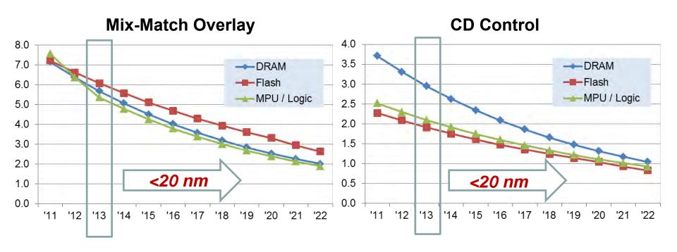
On-going improvements to productivity, overlay, and CD control are essential for future scaling and 450 mm
