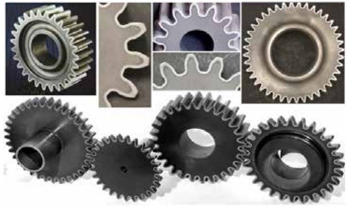
Figure 2: In some cases, a certain hardness gradient can provide a gear with superior performance, although, in many applications, a true contour hardening pattern yields the best gear characteristics. (Courtesy of Inductoheat Inc.)
