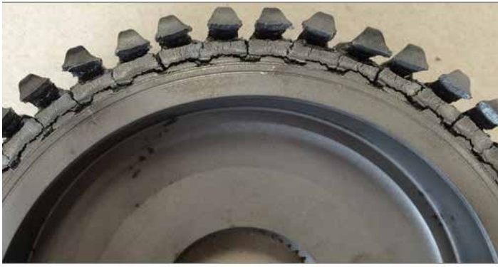
Figure 5: Shown here is an example of applying excessive power density and the use of lower than-optimal frequency.
