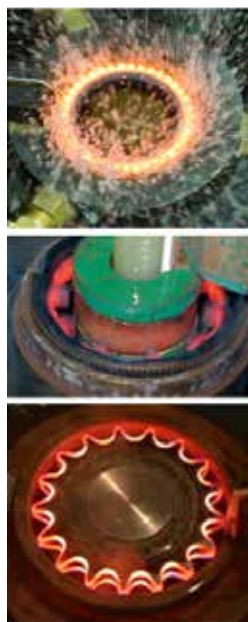
Figure 1: These images show induction gear hardening by encircling the whole gear (external or internal) or sprocket with an induction coil; the so-called “spin hardening.” (Courtesy of Inductoheat Inc.)
