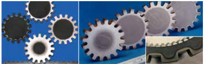
Figure 3: These hardening patterns were obtained on the same carbon steel shaft (left and middle images), with teeth using different combinations of heat time, frequency and power [1].
