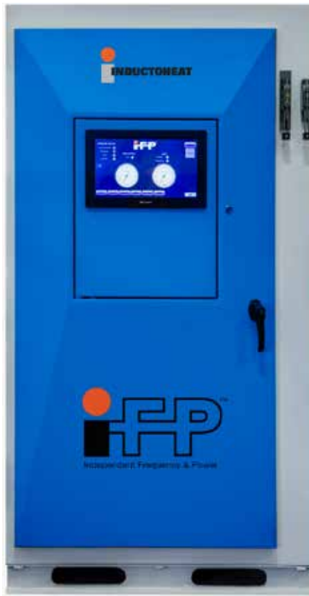
Figure 6: The Statipower IFP inverter (patent pending) has the ability to independently and instantly change both frequency and power during the heating cycle, which allows heat treaters to use a lower frequency for preheating the root areas while a higher frequency helps ensure sufficient heating of the tooth flanks and tips. (Courtesy of Inductoheat Inc.)
