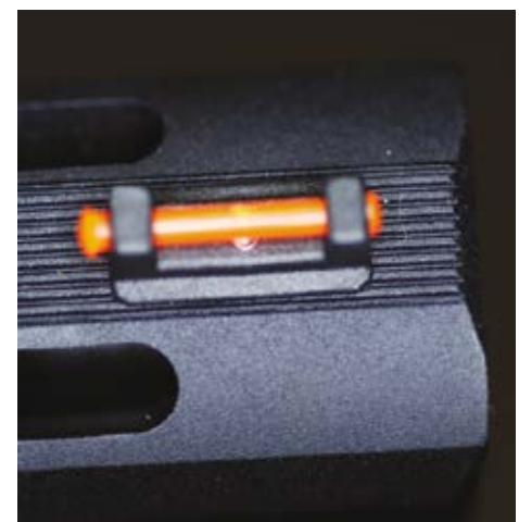
The front-sight includes a piece of high-visibility fibre-optic red plastic.
