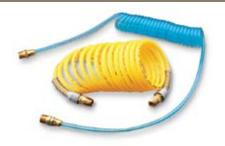
**Ultra-Lite** >>**Superbraid**<**Air Hose** - 63% lighter weight than rubber products. Extremely tough and abrasion resistant. Available as hose assembly with state-of-the-art strain relief system, allowing hose to bend freely without kinking. Up to 220 psi. -40°F to 165°F. Sizes 1/4" - 3/8" I.D. Blue and yellow.
